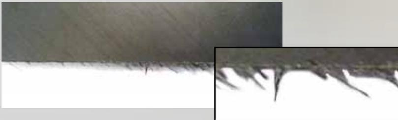
Milled CFRP workpiece edge without delamination machined with a Guhring CR 100 end mill
