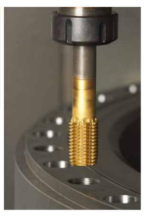
Industrial sectors such as transmission, turbine and energy plant manufacturers require exceptionally large threads. For exactly such applications we have the taps, Guhring nos. 778 and 779 as well as the fluteless tap, Guhring no. 923 in the range for thread sizes M16 to M39.
